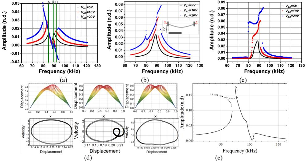
**Fig. 1.** Galerkin Results at (a)  $x=0.5$ , (b)  $x=0.25$ , and (c)  $x=0.75$  ( $x$  denotes the normalized beam position with respect to the beam length). (d) Oscillations of the beam and phase portraits at different sections shown in (a) (A, B, and C from left to right). (e) MTS results of the dynamic response of the arch beam at  $V_{DC}=50V$  and  $V_{AC}=10V$ . The inset of (b) presents a schematic of the arch beam.
