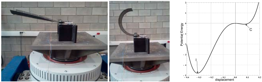
Fig. 2. Multistable shell I-state (a), C-state (b) and function of potential energy with indicated I and C states (c).
