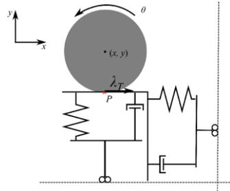
**Fig. 1.** Illustration of the compliant ground model
