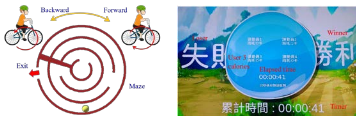
Fig. 2. The maze rotation corresponded to the motion of the tiny aerobic equipment, and the exercise state revealed after playing.
