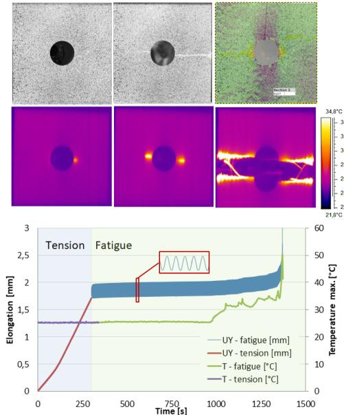
**Fig. 1.** The fatigue test results of the composite plate with hole registered by the infrared thermography and the digital image correlation systems.
