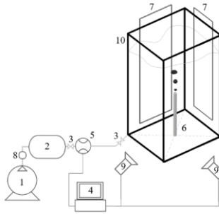
**Fig. 1.** Experimental setup: 1 - compressor, 2 - air tank, 3 - ball valves, 4 - computer, 5 - mass flow meter, 6 - brass nozzle, 7 - led panels, 8 - proportional valve, 9 – double camera system, 10 – glass tank.
