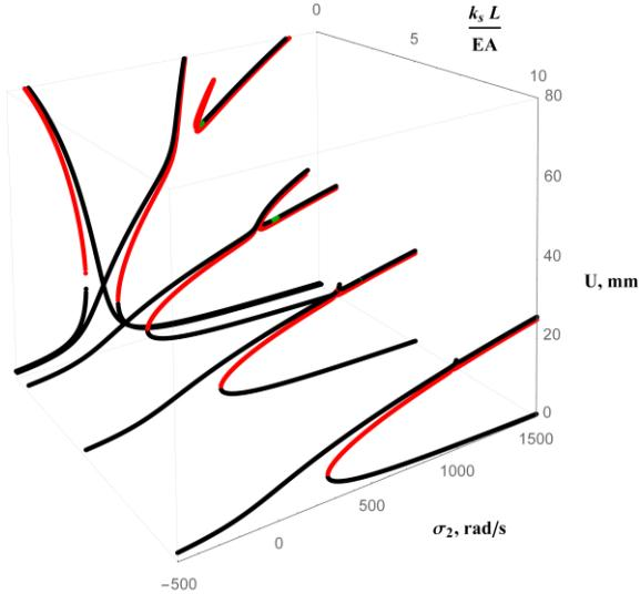
**Fig. 2.** Frequency response curves of the beam-spring system for  $Z=1/4L$  and dimensionless stiffness coefficients  $k_s L/EA$  equal 0, 0.1, 1, 5 and 10 (back to front). Jacoby stability analysis: stable (black), unstable saddle-type (red) and unstable source type (green) solutions.
