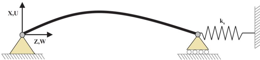
Fig. 1. The beam-spring system
