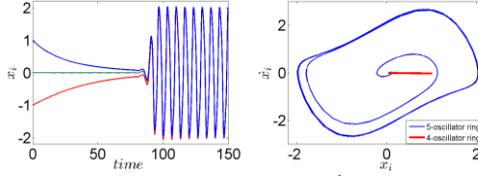
**Fig. 1.** (a) Frequency synchronization due to the presence of a 5<sup>th</sup> oscillator. (b) Limit cycle oscillation in a 5-oscillator ring changes to amplitude death in a 4-oscillator ring.
