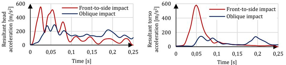
Fig. 2. The course of the vehicle D occupant head acceleration (left figure) and torso (right figure) during a front-to-side and oblique impact
