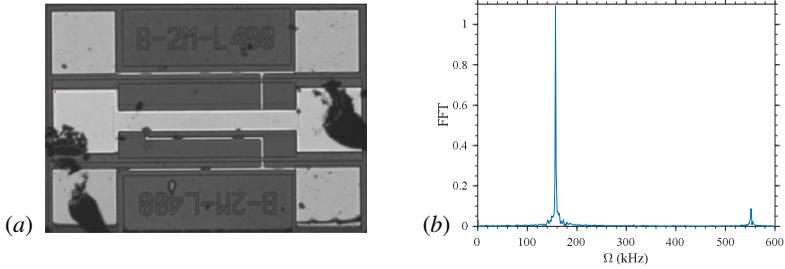
**Fig. 1.** (a) Optical image of the fabricated MEMS device. (b) FFT spectrum of the device experimental response at the internal resonance in the impacting dynamics.
